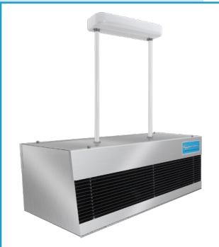
Figure 2 – Shows the top of Hygeaire® Model LIND24-EVO-2PM (above). Note the two mounting holes on the top of this fixture (these are for the Pendent Mount Canopy Set attachment). The fixture is to be mounted at a minimum height of 7 feet from the bottom of the fixture to the floor, in a location that must be able to safely support 32 pounds.
